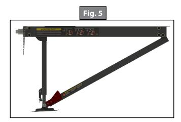
4. Continue to turn the hex coupler clockwise until the footpad touches the ground and resistance is felt.
