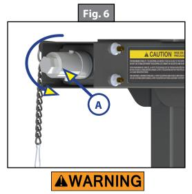
Quick retracting stabilizers can pinch, crush and cut causing severe personal injury. Keep clear and use caution when operating stabilizers to avoid personal injury.
